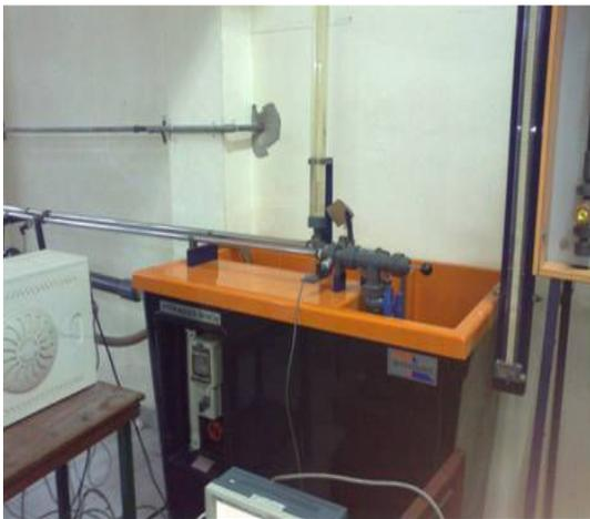
Gambar 2. Hydraulic Bench Apparatus
